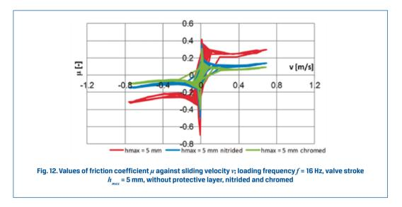
Such courses have quite large width of hysteresis, which is a characteristic property for courses of the close to dry friction coefficient as the function of sliding velocity. Obtained values of mixed friction coefficient are in good agreement with measured values of dry friction coefficient. The highest values have been for non-coated valve stem and the lowest for the chromed one.
