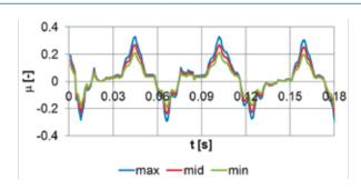
Fig. 8. Calculated values of friction coefficient  $\mu$  between valve and its guide against time t; loading frequency f = 16 Hz, valve stroke  $h_{max}$  = 5 mm
