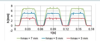
Fig. 4. Measured valves of the valve lift h against time t; loading frequency f = 16 Hz, valve stroke  $h_{max}$  = 7 mm,  $h_{max}$  = 5 mm, and  $h_{max}$  = 3 mm, respectively
