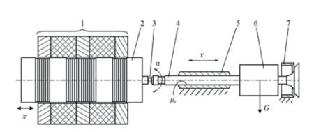
Fig. 3. The model of the assembly consisted of movable coil the drive and valve bearing in its guide and loaded by additional weight; 1 - immovable part of the drive, 2 - movable coil, 3 - spherical joint, 4 - valve, 5 - guide, 6 - additional weight, 7 - seat insert
