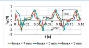
Fig. 7. Measured values of the friction force  $T_R$  between valve and its guide against time t; loading frequency f = 16 Hz, valve stroke  $h_{max}$  = 7 mm,  $h_{max}$  = 5 mm and  $h_{max}$  = 3 mm, respectively,  $T_{max}$  – maximum friction force during valve displacement against its guide
