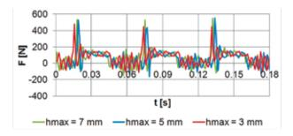
Fig. 6. Measured values of the impact force F between valve and its seat insert against time t; loading frequency f = 16 Hz, valve stroke  $h_{max}$  = 7 mm,  $h_{max}$  = 5 mm and  $h_{max}$  = 3 mm, respectively
